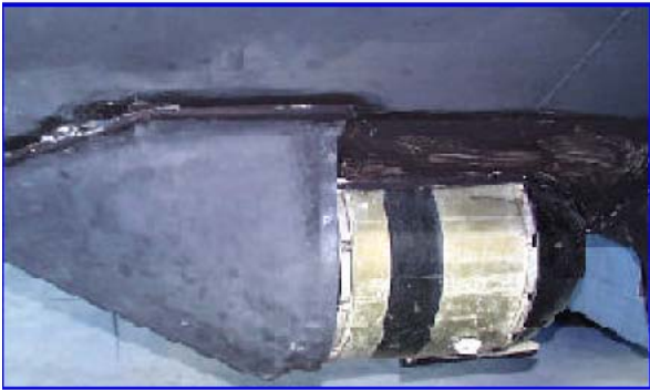
Multibeam sonar head RESON SeaBat 8101, mounted on Survex1 (SMF Europe survey vessel)
